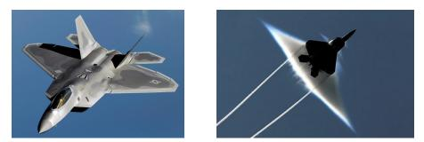
3. At the edge of a shock wave (picture above on right), pressure nearly has a jump discontinuity.
