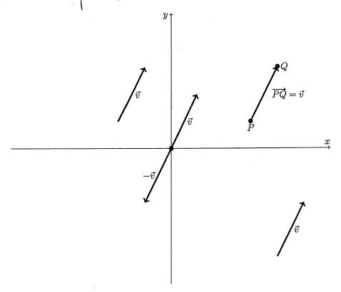
We often write a vector with an arrow over a letter to distinguish a vector  $\vec{v}$  from a scalar v, but we also can talk about the vector between two points P and Q, denoted  $\overrightarrow{PQ}$ .
