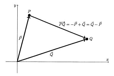
If we know the components of the points involved, then we can compute the components of the vector  $\overrightarrow{PQ}$ . For example, if we want the vector from P(1,3,-1) to Q(-2,0,3), then we compute
